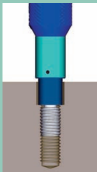
Reduced diameter for counterbores.
