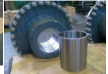
Conical sleeve for hydraulic dismounting
