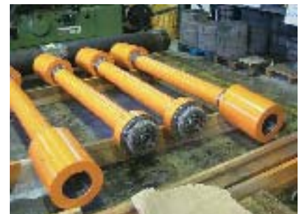
Skin Pass gear spindles
