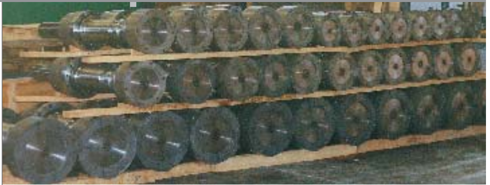
Complete wire mill spindles.
