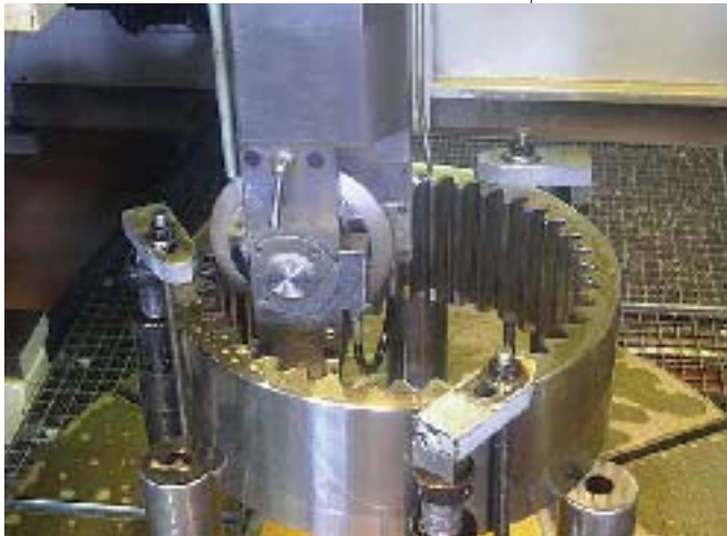
Internal sleeve grinding.
