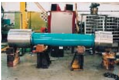
Hot strip mill spindle at maintenance
