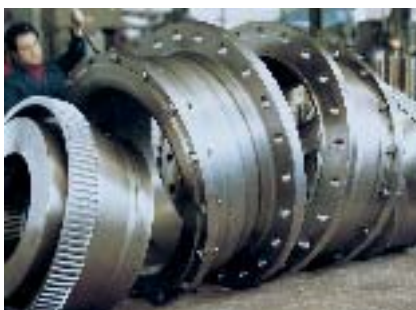
Main Drive Gear Coupling
