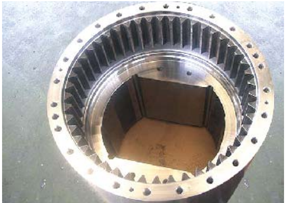
Carburized coupling box.
