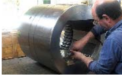
Coupling Box deburring
