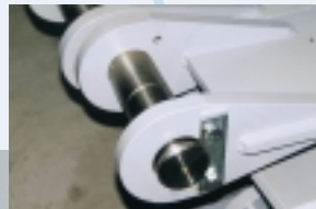
A drive unit with an auxiliary drive for a leca bebble dryer drum.
