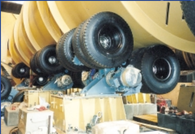
Special gear units for a rubber tyre supported debarking drum.
